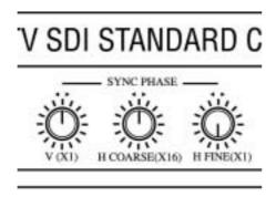
Factory-shipped SYNC PHASE settings: The machine should be normally used with these settings.
